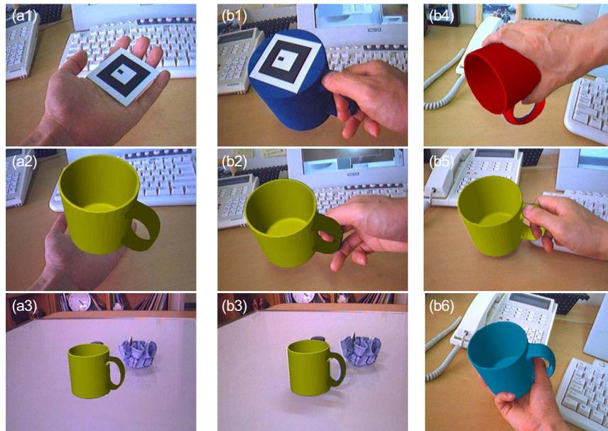
**Figure 3.** General-purpose AR (a1~a3) and Augmented Foam (b1~b6): (a1) Plane marker (a2) Virtual overlay on a plane marker (a3) Virtual overlay on a table, (b1) Augmented Foam without virtual overlay, (b2) Augmented Foam with virtual overlay (visibility problem), (b3) Augmented Foam on a table, (b4~b6) Augmented Foam with corrected hand visibility (various color cups)
