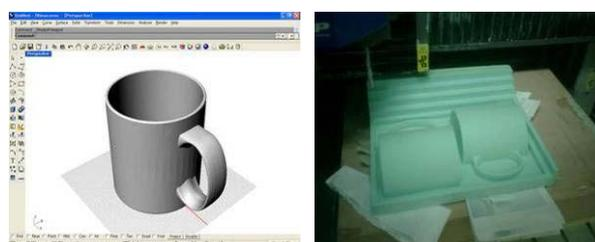
Figure 2. Process of constructing Augmented Foam: 3D CAD modeling (left) and CNC-produced foam mock-up (right)
