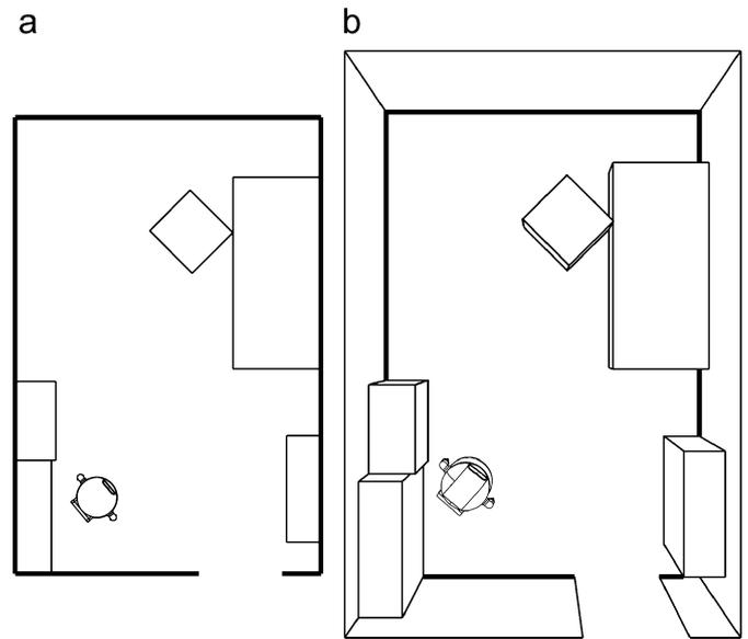
Fig. 9. Dimensionality of the map. (a) Two-dimensional representation; (b) the elevated two-dimensional ( $2_{1/2}$ ) representation.
